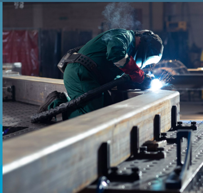
Box section steel welding Image courtesy of Hutchinson Engineering. All rights reserved.
