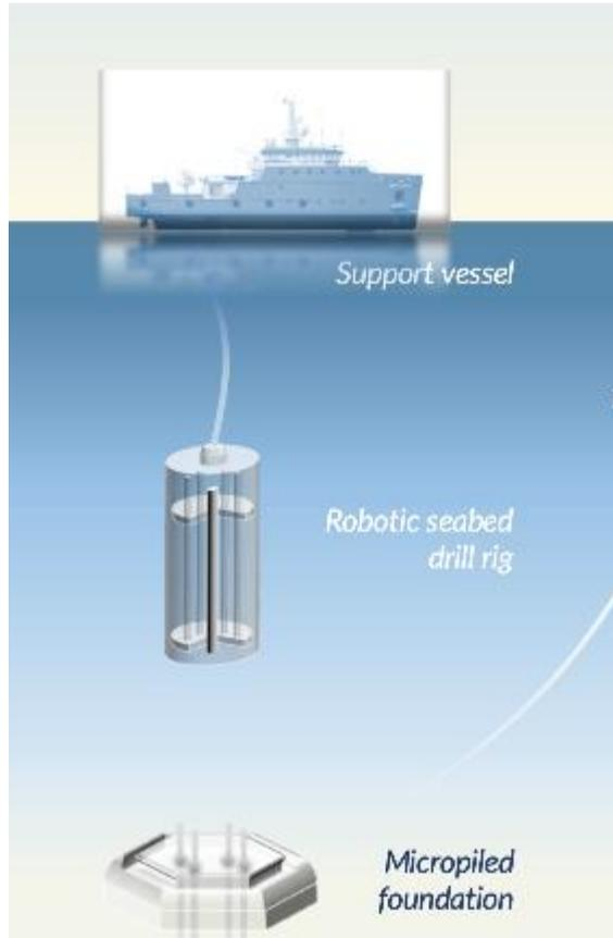
Install micropile anchors offshore (with load test)
